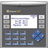
Pressing F1 initiates the zero and span cycle. The cycle will be in Zero for 3 minutes then Span for 3 minutes and return to normal operation automatically.
